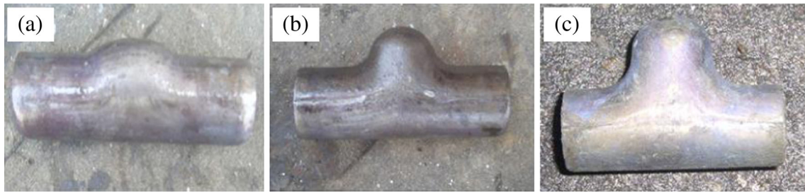
Fig. 11 Forming results in three steps: a the first step, b the second step, and c the third step
