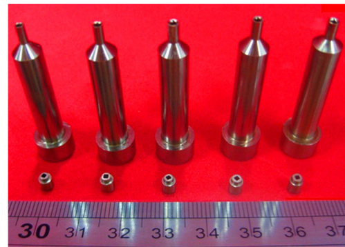
Fig. 2 Compound punch-dies and blank holders
