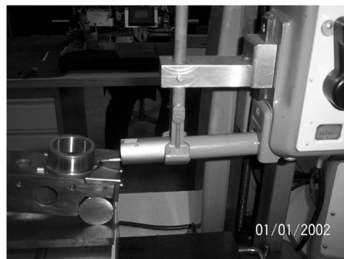
Fig. 2 Measurement of roughness on the supporting face of inner ring of the bearing with tapered rollers
