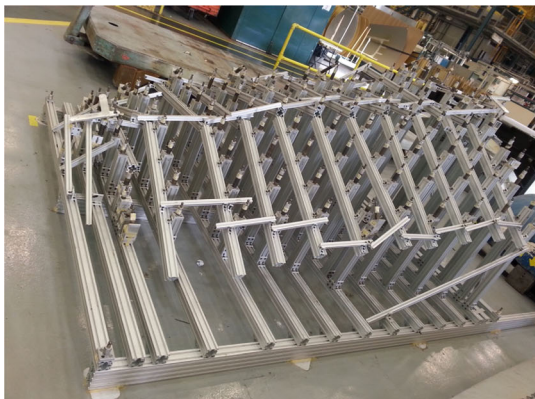
Fig. 1 A special, expensive, heavy, and complex fixture for the inspection of a flexible plate, Bombardier Aerospace Inc. Left the fixture without the part, right the CAD model of the fixture with the part set up on it
