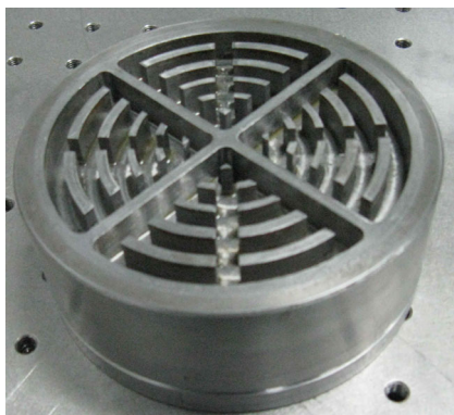
Fig. 11 The mold surface in elastic deformation machining
