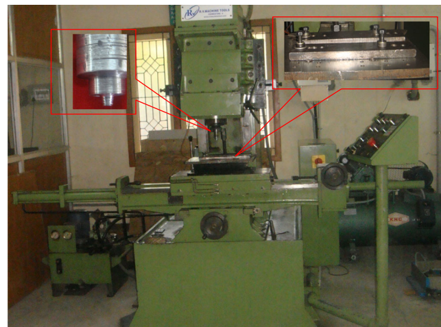
Fig. 1 Photograph showing experimental setup of FSW machine
