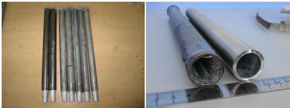
Fig. 1 CLAM steel/aluminum bimetal tube prepared by explosive welding
