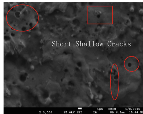
(c) SEM images about surface crack of SCD in Table 9 using BPNN-GA optimization
