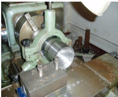
Fig. 4 Face cutting experiments on sleeve parts
