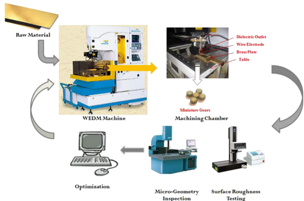
Fig. 10 Tasks performed for mesofabrication of quality gears by WSEM [18], ©2014 Taylor and Francis LLC
