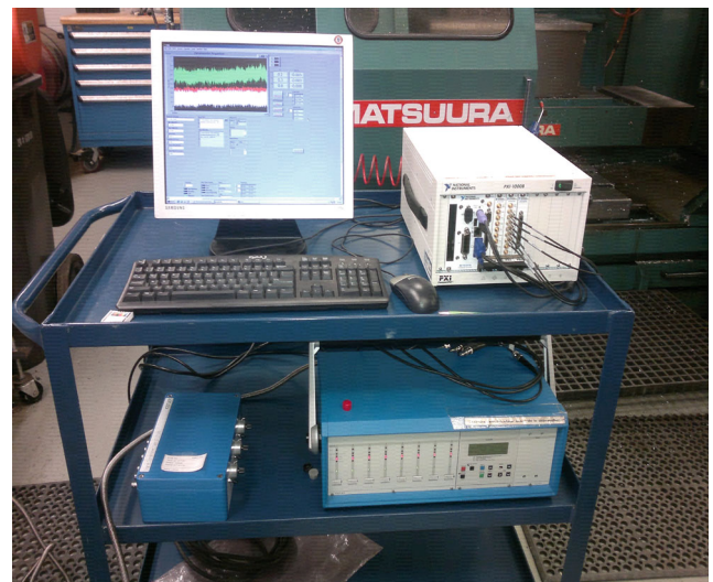
Fig. 6 LabView based data acquisition system with Kistler dynamometer
