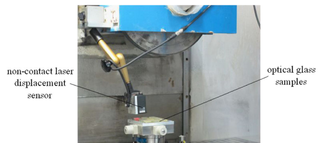
Fig. 5 Onsite measurement of optical glass samples
