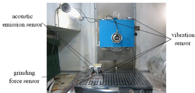
Fig. 4 Installation methods of all sensors and experimental panorama
