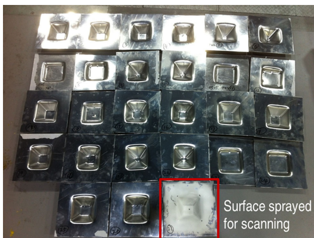
Fig. 6 Truncated pyramids by incremental sheet forming
