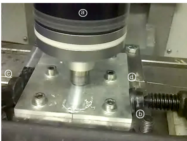
Fig. 1 FSW device (a) and test fixture (b) with two embedded thermocouples (c) and (d)
