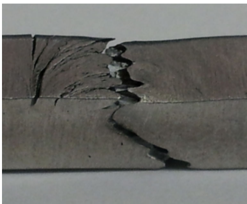
Fig. 18 Fracture zone under the tool pin using sample 2n with the lowest average axial force; notice the delaminated regions in vicinity of the weld line
