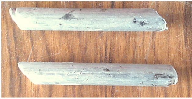
Fig. 6 Aluminum specimens after one pass of ECAP process
