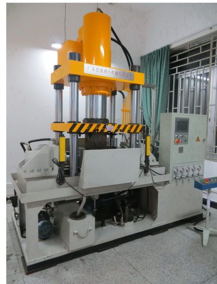
Fig. 9 The CNC Tube Hydroforming system YB98-200A (made in China) was applied to conduct the hydroforming experiments
