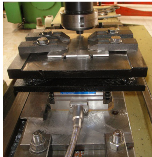
Fig. 2 A view of the preparation of friction stir welding process
