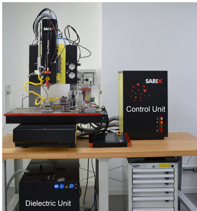
Fig. 1 Sarix SX-200 micro EDM milling machine used in the experiments
