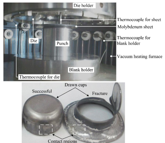
Fig. 5 Test device for vacuum hot deep drawing of pure molybdenum sheet
