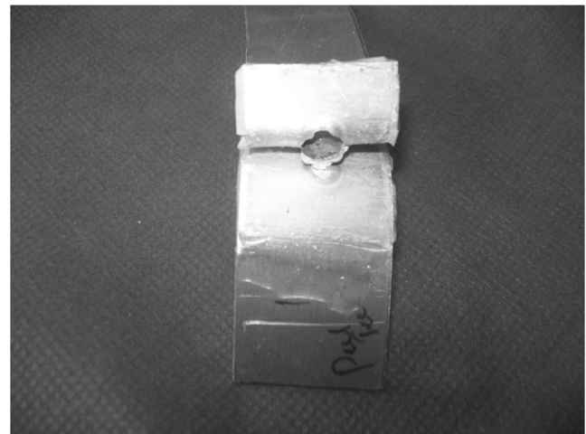
Fig. 18 Tear test of a weld-bond specimen
