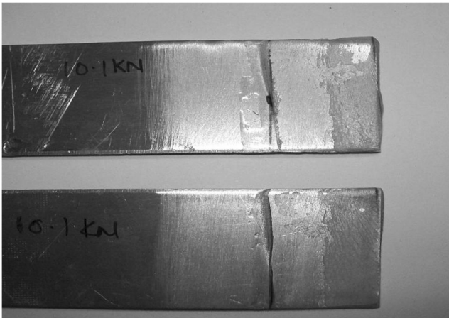
Fig. 5 Adhesive bond joint after tensile testing (cured at 120 °C for 60 min)
