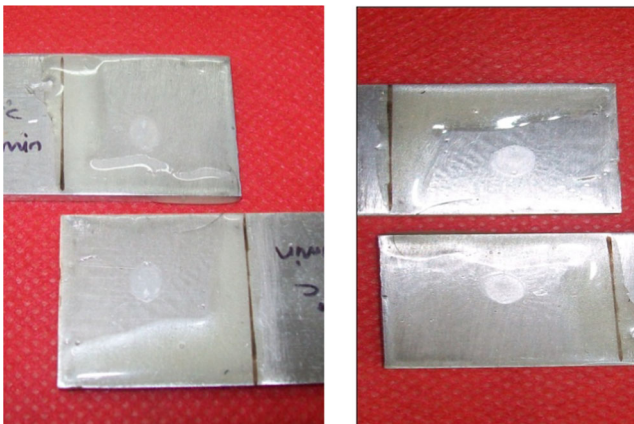
Fig. 24 Un-welded weld-bonded specimen
