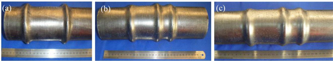
Fig. 14 Wrinkle behavior for the welded tube during hydroforming: a 2.5 MPa, b 3 MPa, and c 4.5 MPa
