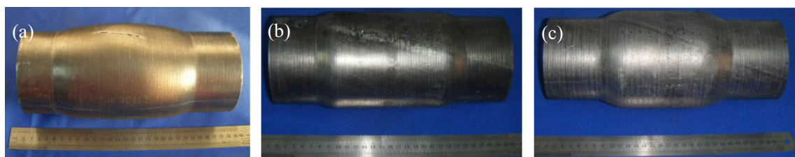
Fig. 4 The part formed by hydroforming: a typical fracture appearance of the FSW tubes, b the preformed part with a expansion ratio of 10 %, and c the finish part with a expansion ratio of 20 %
