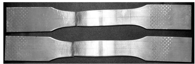
Fig. 11 Failure location in the weld tension test
