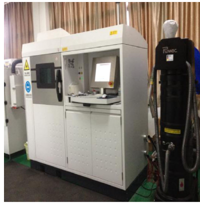
Fig. 4 The DMSL equipment of EOSINT M280 and the manufacturing schematic diagram
