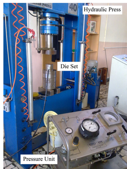
Fig. 7 Photograph of the experimental forming setup
