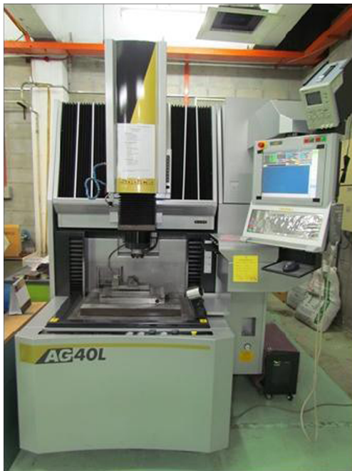
Fig. 1 AG40L Sodick electrical discharge machine
