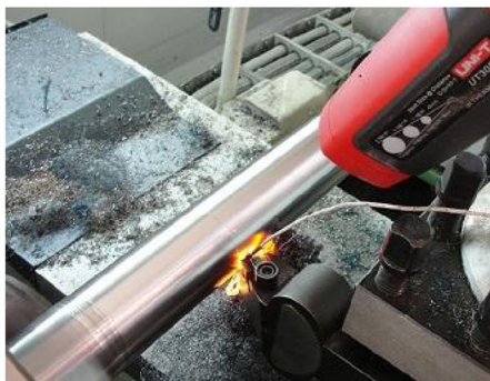
(b) Testing ground of the temperature measurement
