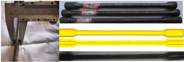
Fig. 16 Experiment and simulation of CWR hollow valve
