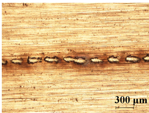
Fig. 8 The results of laser marking pattern using the step and scanning method
