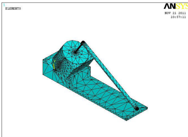
Fig. 6 Finite element model of the motor assembly
