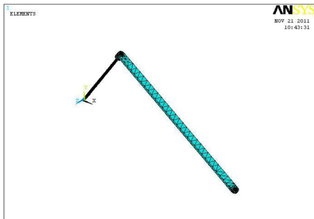
Fig. 10 Finite element model of the crank and shaft subassembly
