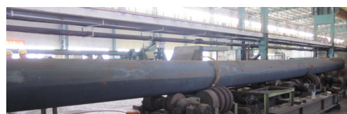
Fig. 3 Measuring site of the straightness-offgrade LSAW pipe
