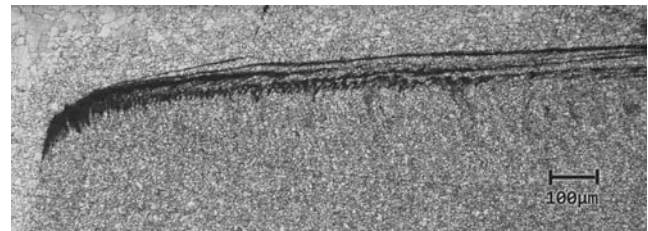
Fig. 14 Apparent defects caused by a hexahedron tool
