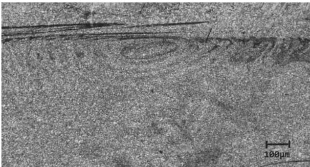
Fig. 13 Formation of onion rings on the top part of the stir zone using a hexahedron tool
