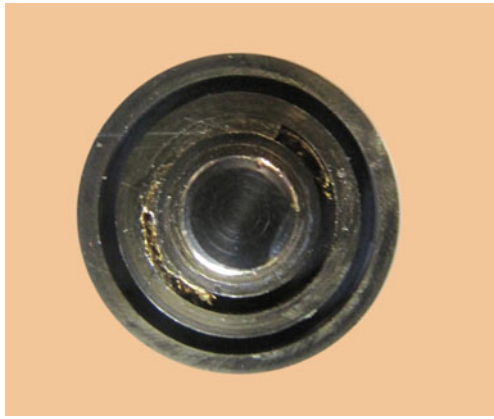
Fig. 4 Brass sticking into shoulder grooves
