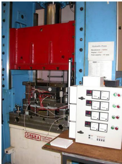
Fig. 14 160-Ton hydraulic press for carrying out warm forming experiment
