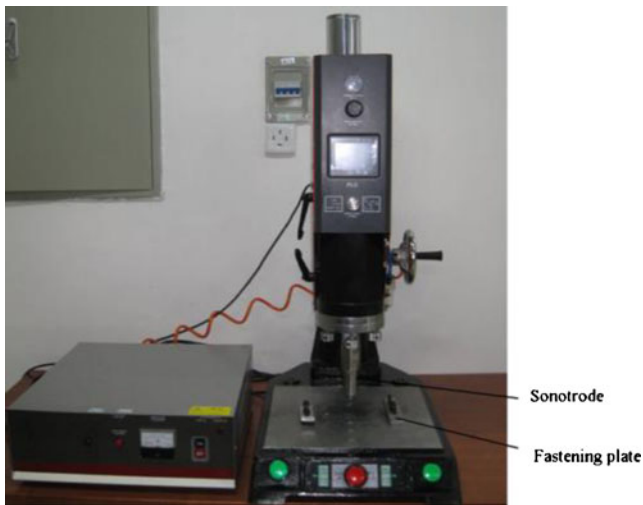
Fig. 2 Ultrasonic plasticizing and molding experimental platform
