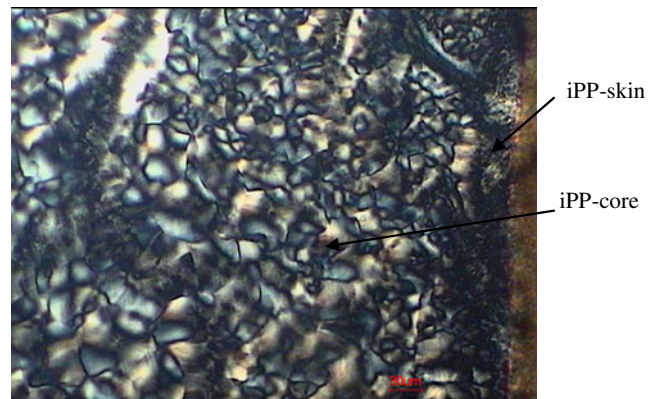
Fig. 9 Polarizing microscope photo of PP plastic parts
