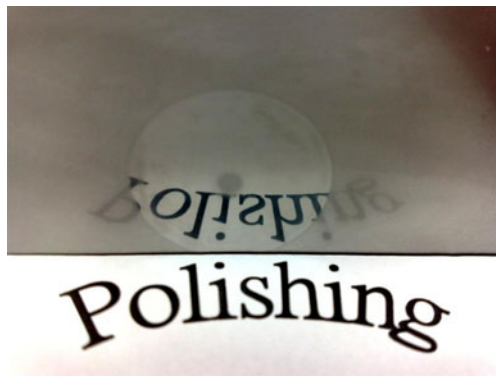
Fig. 9 Surface with mirror reflection achieved by 2D-VAMAF
