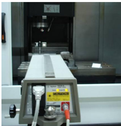
Fig. 9 Measuring positioning errors by using laser interferometer
