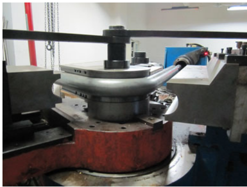
Fig. 8 NC hydraulic tube bender W27YPC-159 and the formed QSTE340 welded tube
