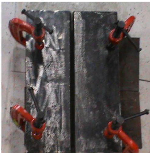
Fig. 2 Specimens used for welding with their assembly
