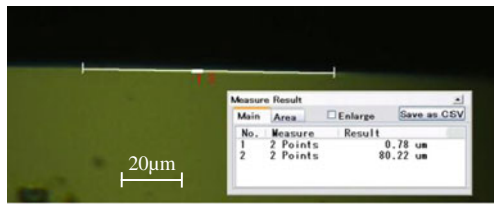
Fig. 14 Tool wear of diamond cutting plasma nitrided NAK80 using CAMQL system after a cutting distance of 150 m [36]
