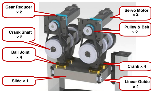
Fig. 4 Slide driving system
