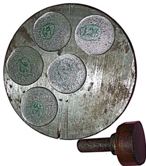
Fig. 2 Copper electrode and AISI D2 workpiece
