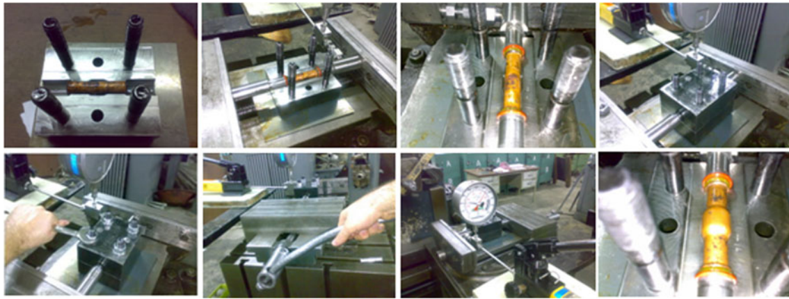
Fig. 4 Sequences of experimental tube hydroforming tests
