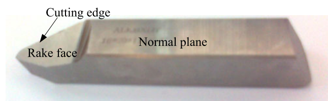
Fig. 2 Face milling blade in industrial application
