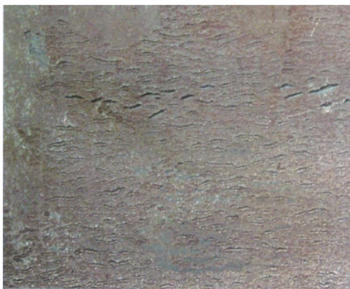
Fig. 13 Surface defects in a strip after hot rolling
