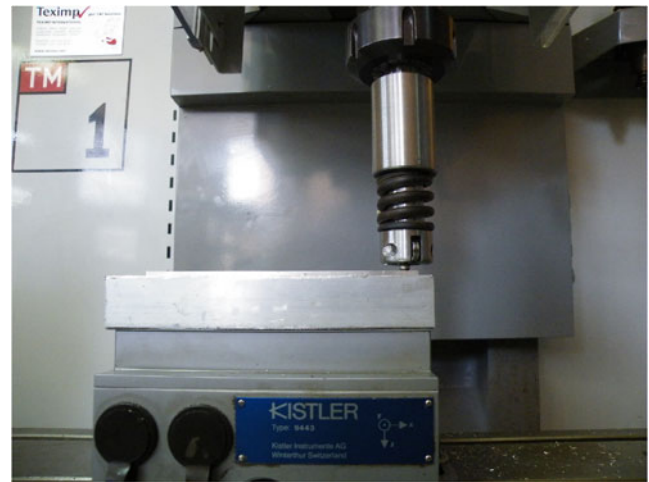
Fig. 8 Photo-image of the redesigned tool system during the process of burnishing
