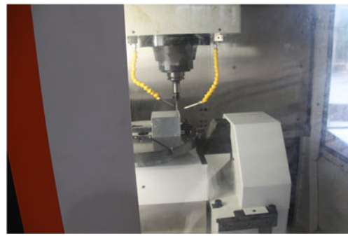
Fig. 4 Machining tests of five-axis machine tool C-axis
