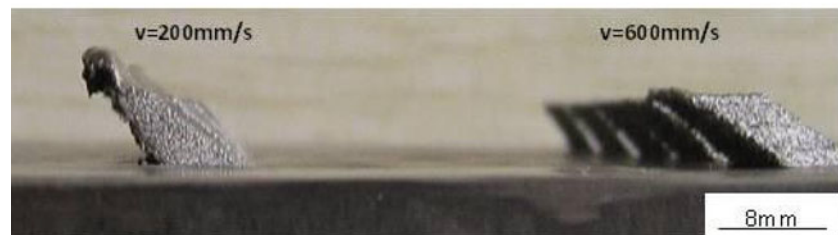
(c) side view of the overhanging surfaces fabrication
