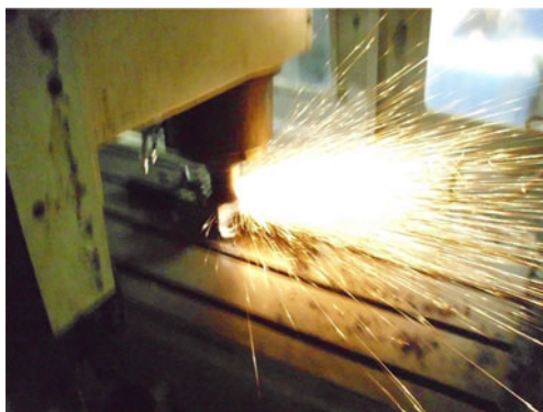
Fig. 17 Photo captured during the milling process ( v=1,200 m/min, f_z=0.1 mm/tooth, a_p=0.3 mm)
