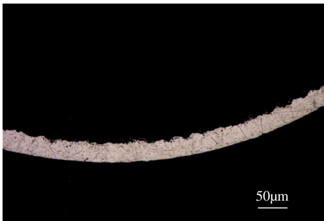
Fig. 4 Micrography of the continuous chip ( V=100 m/min)
