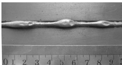
Fig. 12 The weld bead morphology in GMAW ( \nu_w=1.30 m/min, I=321 A, U=30 V)
