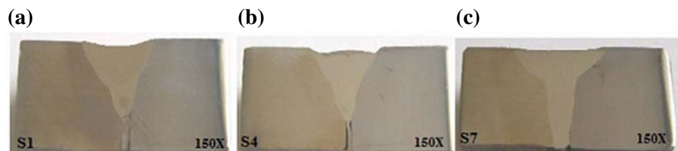
Fig. 5 The cross-sectional macroappearance of KPTA-welded specimens. a S1, b S4 and c S7 specimens
